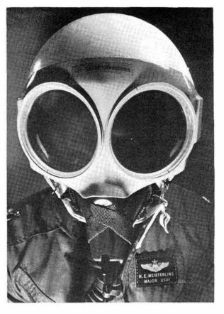
HOW'D you like to meet this character on a dark night? It's not likely unless you take up flying with the Air Force. He's wearing Sandia's thermal and flash protection goggles, whose lenses are made of PLZT ceramic. Goggles prevent blindness from flash of nuclear burst.
